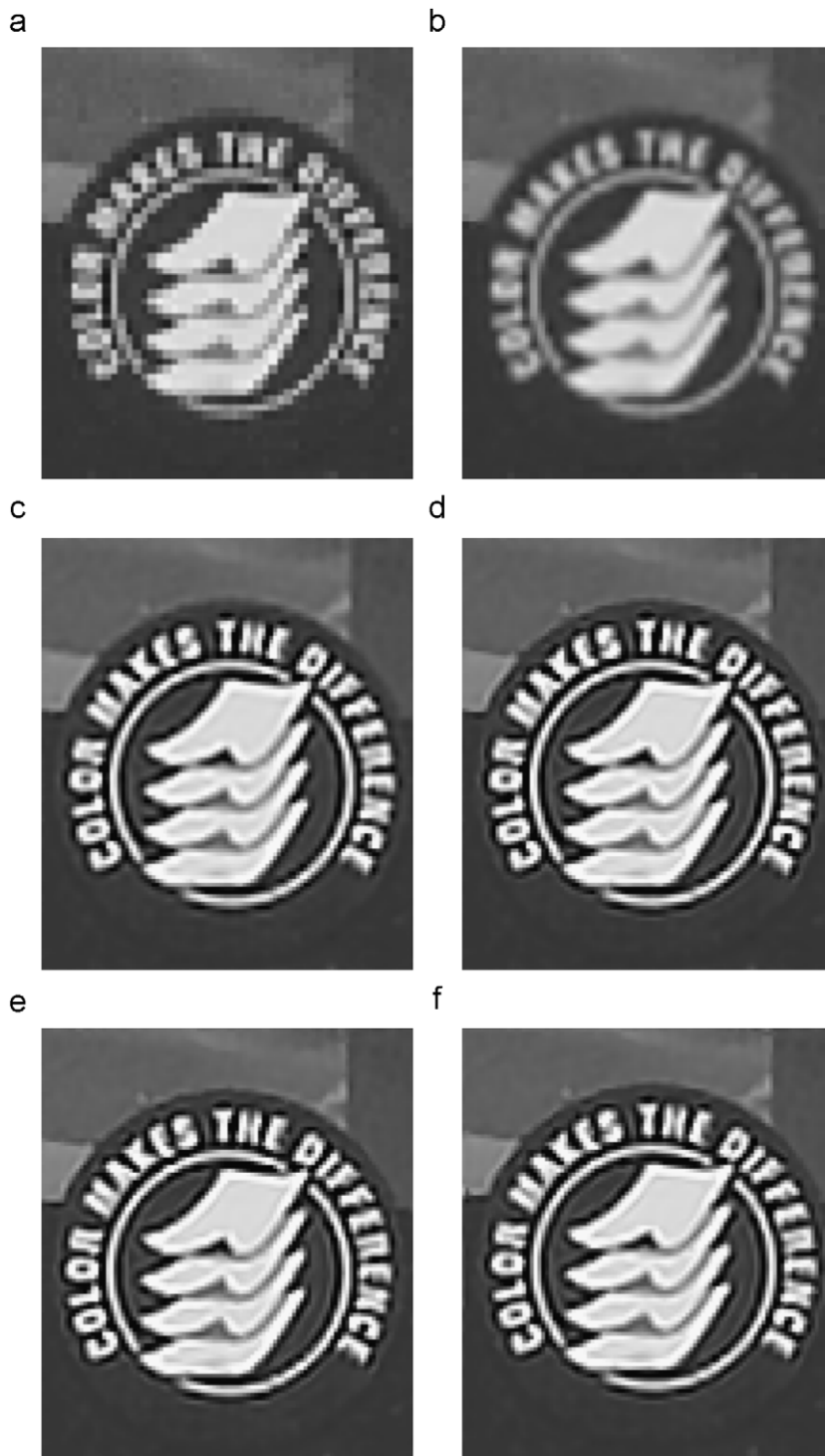
Fig. 9. Results of super-resolution reconstruction using different regularizations. (a) Frame 1 of the surveillance sequence. (b) Bilinear interpolation. (c) SR result with HMRf regularization. (d) SR result with HWMRF regularization. (e) SR result with HWMRF regularization of frame 3. (f) SR result with HWMRF regularization of frame 5.
